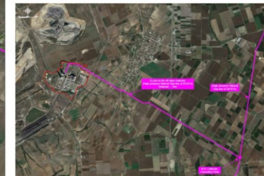
Project layout illustrating the required 7 km pipeline to link the electrolysis plant with the DESFA NG pipeline
